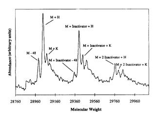
Figure 1. The reconstructed molecular weight plot obtained from ESI-MS analysis of APH(3')-IIa modified by compound 4, and the relevant peak assignments. ESI-MS was performed on a PE Sciex API-III (Ontario, Canada)
